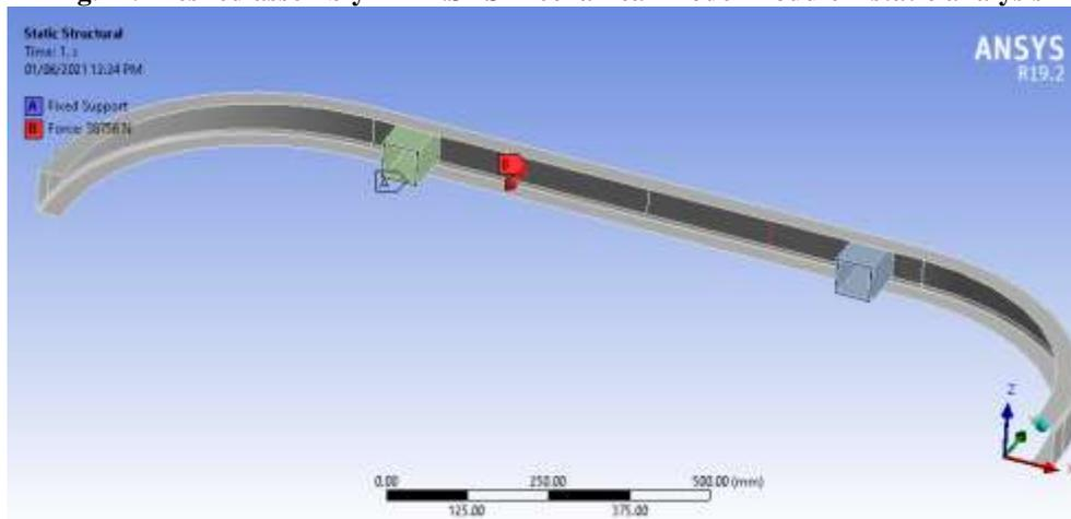
**Fig. -3:** Simulation condition in ANSYS Static Structural module
