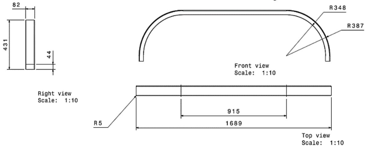
**Fig. -1: Dimensions of the bumper beam**
